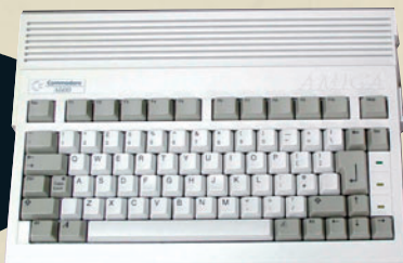
» The lack of a numeric keypad made the low-level Amiga A300/A600 incompatible with several software packages.
